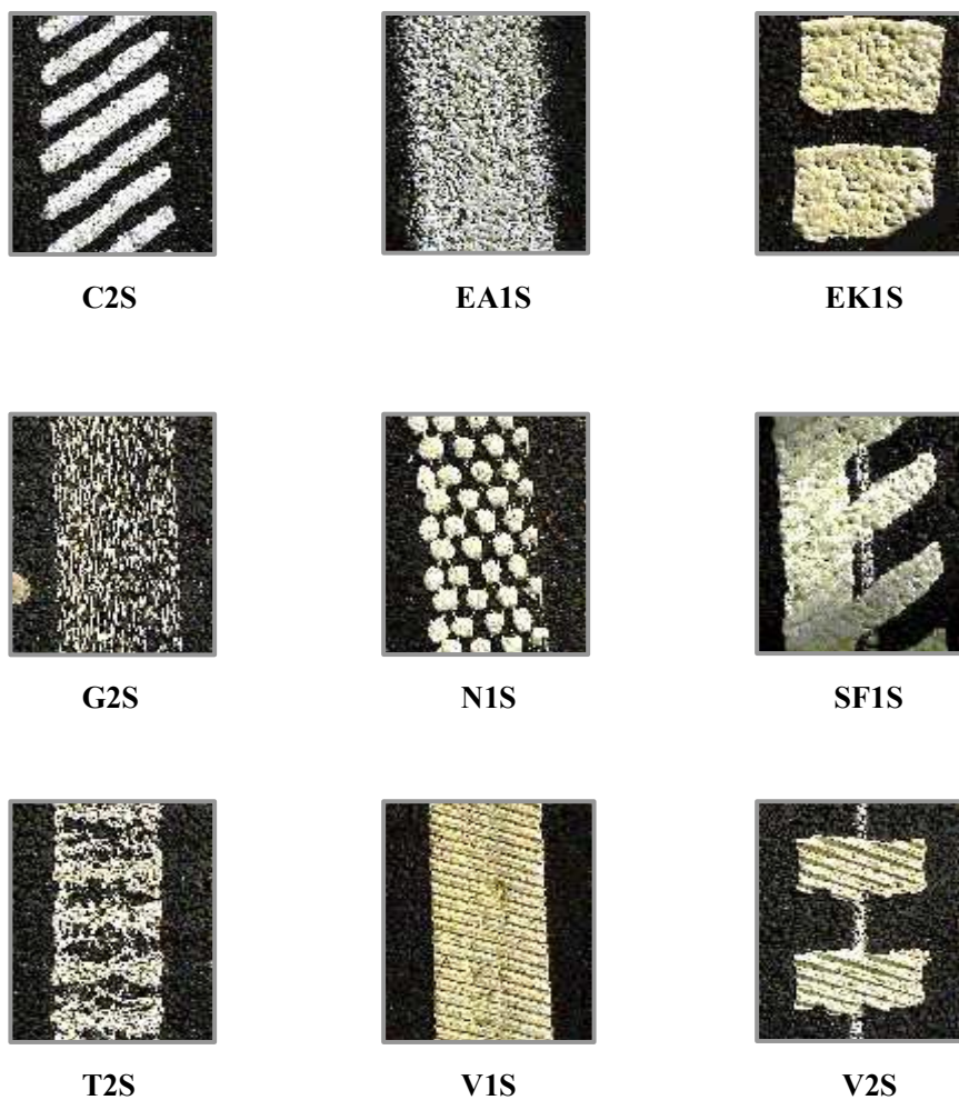
Figure 4 A selection of the test markings on Road 63. This is a representative selection of the different types laid on both test roads. Photographer: Timo Unhola, VTT, Finland.
